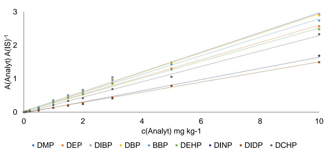
The calibration was automatically spiked and measured. It is an external calibration in acetonitrile.
