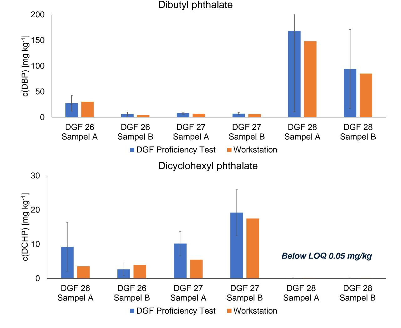
The reference material was prepared according to the draft ISO CD TS 16465 for the determination of phthalates in animal and vegetable fats using the Workstation Phthalates and measured on a GCMS. Only values for dibutyl phthalate and dicyclohexyl phthalate were available for the reference material. The bars on the results of the reference oils indicate the 2 z-score.
