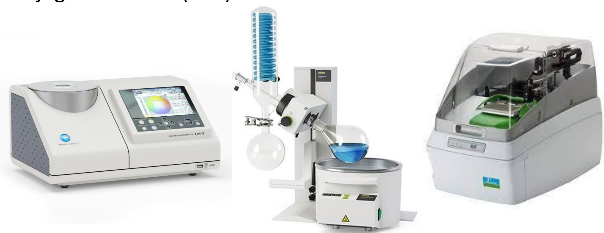
Fig. 2. Konica Minolta CM-5 spectrophotometer, rotary evaporator Rotavapor® R-300, BÜCHI Labortechnik AG and Differential scanning calorimeter DSC 8500
