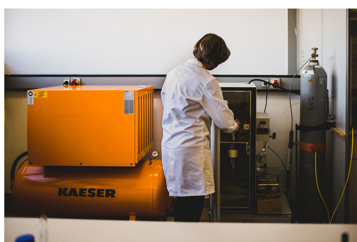
Fig. 2 - SFT-150 scCO 2 extraction system
