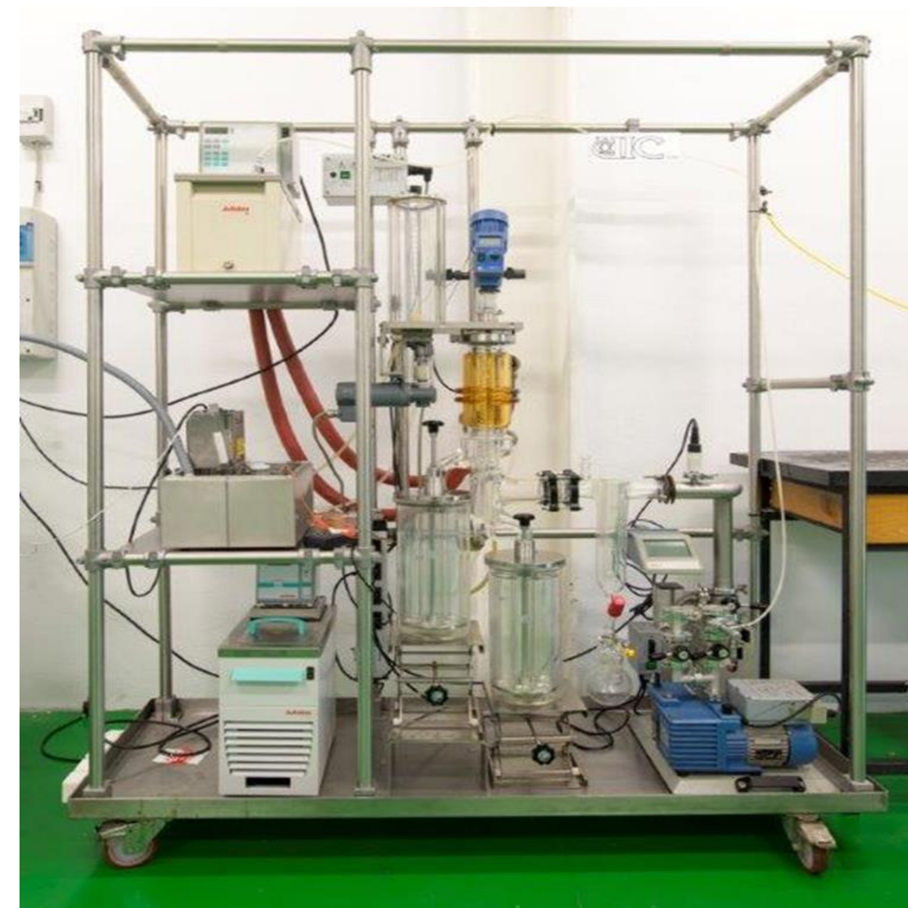
Short-Path Distiller KDL-5 (UIC) • Evaporator area, 4.8 \times 10^{-2} \text{ m}^2 • Condenser area, 6.5 \times 10^{-2} \text{ m}^2
